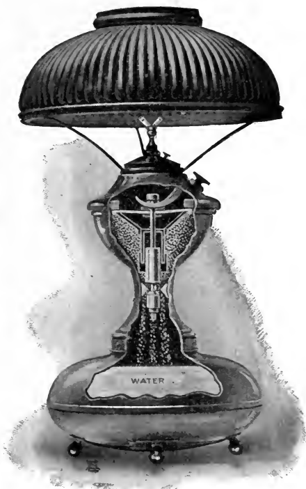
FIG. 105.—Sectional View of the Beck-Iden Acetylene Lamp.
