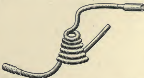
FIG. 29.—Laboratory Copper Coil for Superheating Steam.
