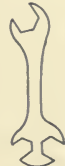
FIG. 2 Wrench for turning off and fastening the Main-Cock in the Gasconducting pipe.
