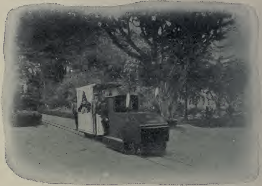
FIG. 147.—Passenger Railway at Exposition Park, Lima, Peru. Equipped with the Deutz Alcohol-locomotive.
