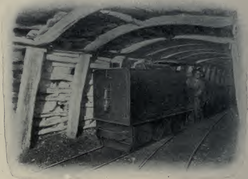
FIG. 145.—Mining Railway of the Krupp Collieries "Hannover" and "Hannibal," Westphalia. Equipped with the Deutz Alcohol-locomotive.
