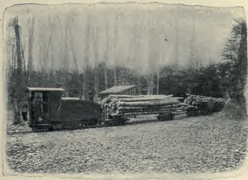
FIG. 146.—Forest Railway of the Grand Ducal Hessian Chief-Forestry in Kelsterbach Equipped with the Deutz Alcohol-locomotive.
