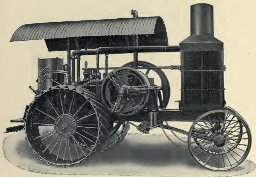
FIG. 152.—Gasoline Traction- or Plowing-engine. Built by the Hart-Parr Co., Charles City, Iowa. This engine can be easily adapted for use with alcohol.
